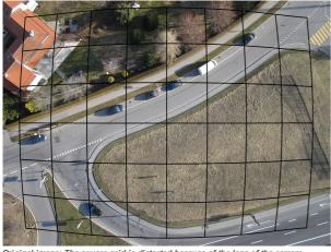
Original image: The square grid is distorted because of the lens of the camera
