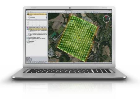
Preview an area of interest, monitor flights in real-time in complete 3D, and modify plans mid-flight. A quality check function verifies data in minutes while you're still on site, indicating sufficient overlap in green.
